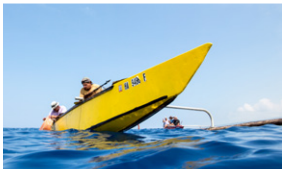
The Pakalana , a bright yellow canoe made of plywood and other easily available material like pipes and driftwood. The ‘ōpelu canoes are designed specifically for fishing, and have a wider hull with storage space for a cooler under the seats and the net along the gunwale. - Photo: Kaipo Kī‘aha
