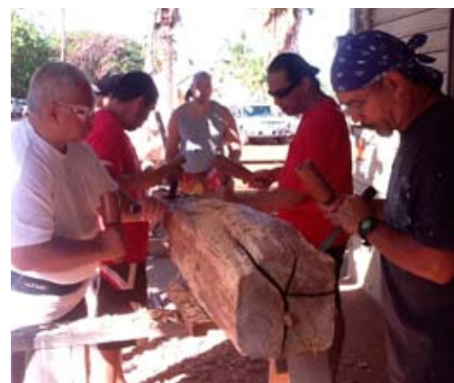
Keoki Ki'ili of Maui, left, and Keoki Makaweole of Kaua'i, right, wielded mallets on ko'i, or adzes, at the Lahaina Carvers Symposium. They are shaping a log into a standard.
